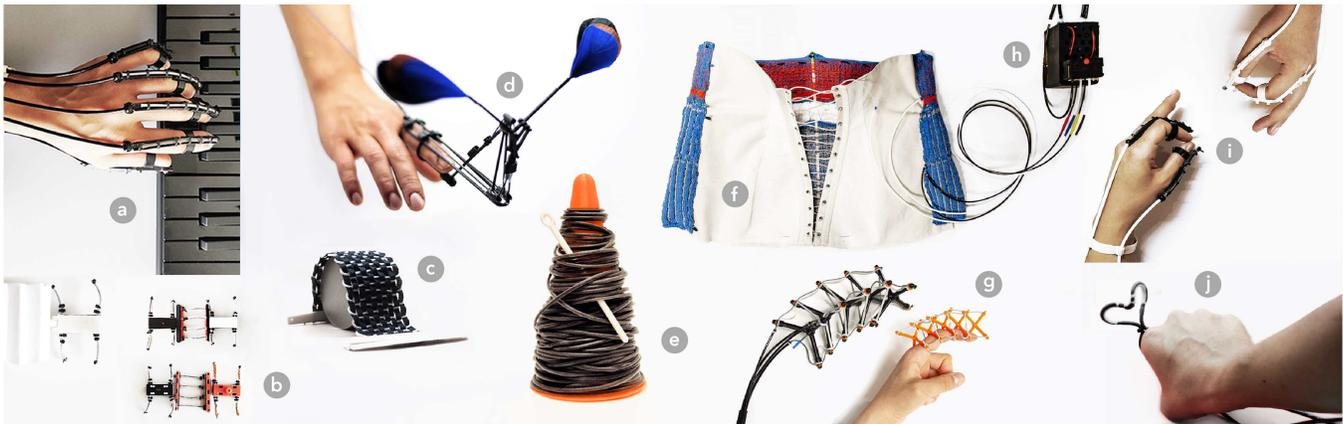
**Figure 1: Omnifiber in use:** (a) An assistive flexoskeleton for piano learning. (b) Patchbot. (c) A woven swatch with Omnifiber. (d) Finger-worn kinetic jewelry. (e) 30 meter Omnifiber spool. (f) Interactive corset inlay-knitted with Omnifiber. (g) Synchronized spine tensegrities with active Omnifiber tendons. (h) FlowIO hardware. (i) Wearable sign language. (j) Heart-shaped dynamic ring.
